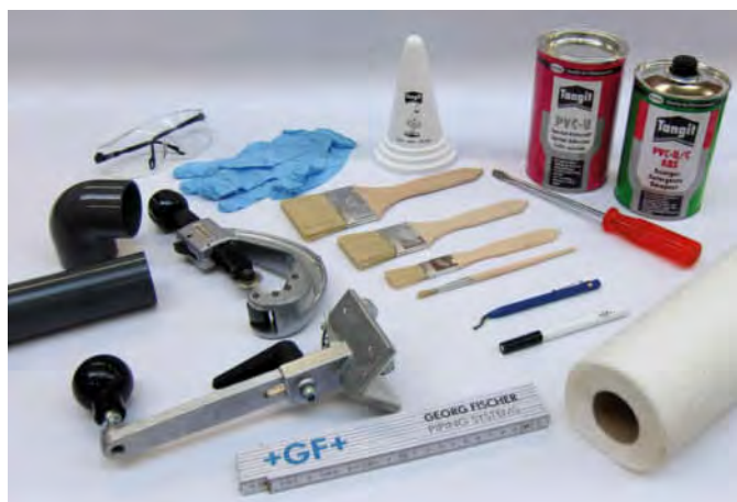
Solvent cementing equipment
