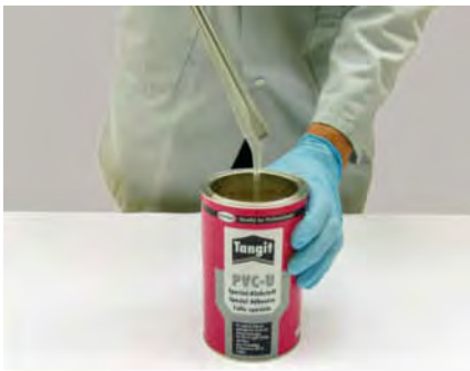
Checking the cement
