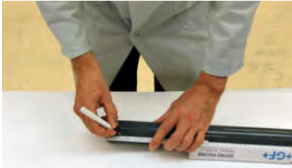
Marking the jointing length
