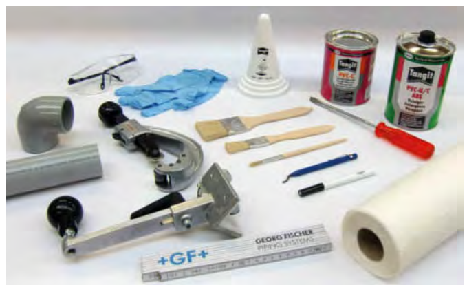
Solvent cementing equipment
