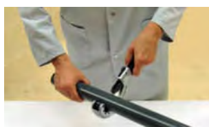
Cutting the pipe to length
